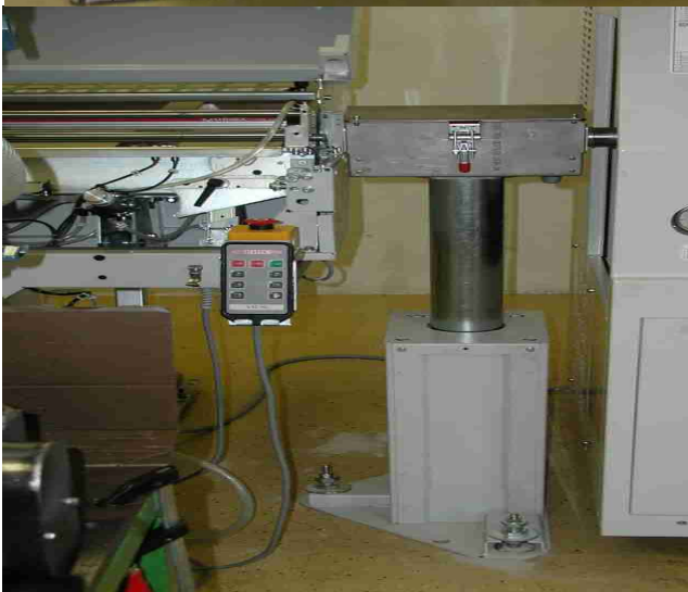
Extern spindle support with bearings
